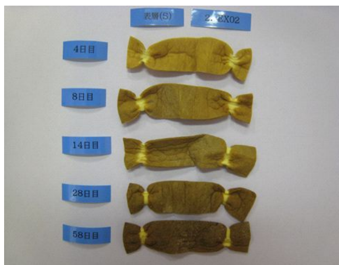
Fig. 4 Uranium adsorbent components after submersion in seawater: the original white color turned brown by adsorption of elemental ions dissolved in seawater.
