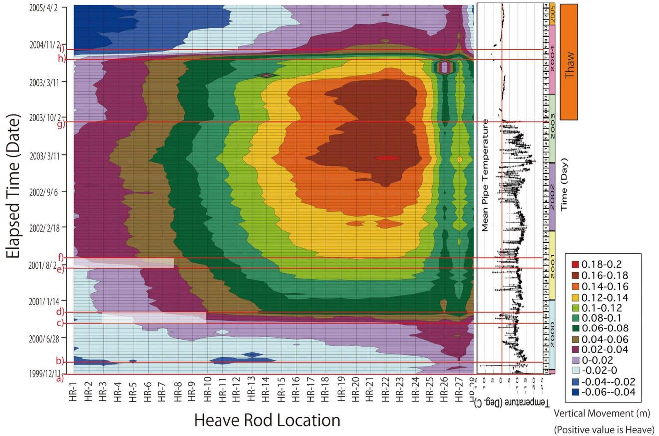
Fig.10 Vertical movement of test pipeline in freezing and thawing phases
