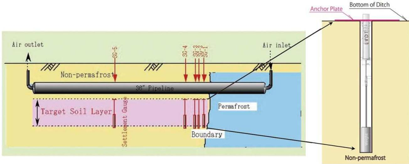
Fig.6 Locations of LVDTs in pipe foundation
