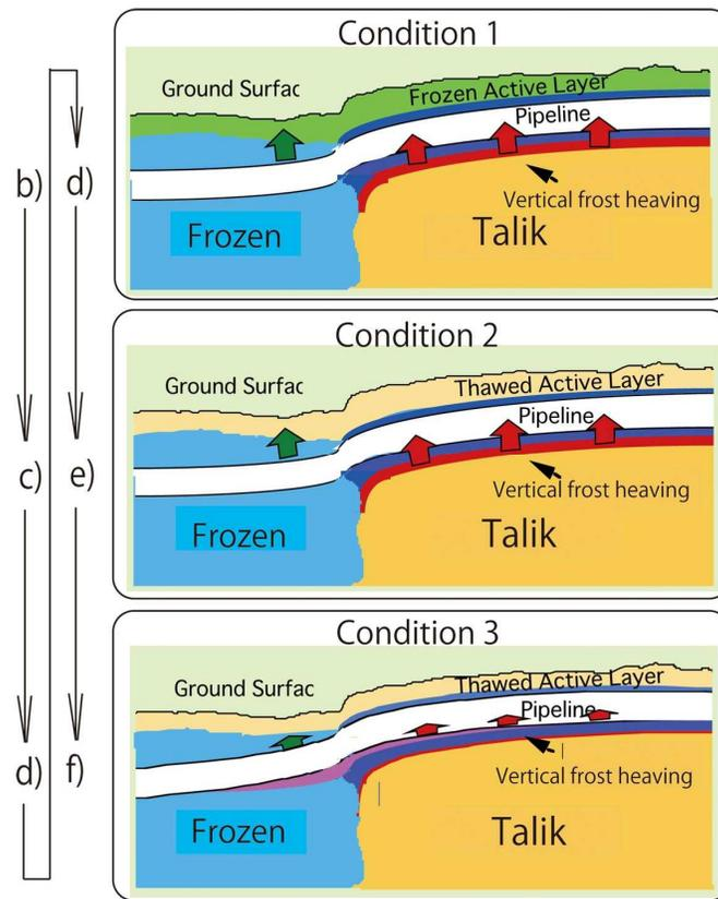
Fig.11 A proposing sequence of ablapt pipeline uplift
