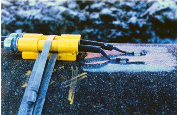
Fig.7 Welded strain gauge
