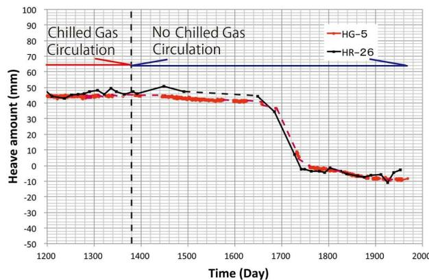
Fig.12 Vertival pipe movement and foundation Settlement during thawing
