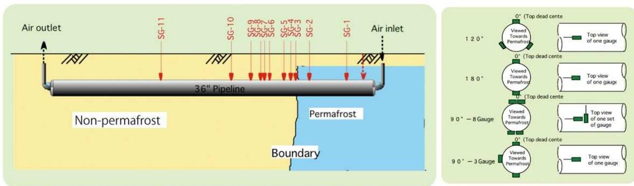
Fig.8 Locations and configurations of the strain gauges
