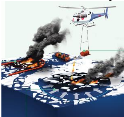
Fig.7 Illustration showing controlled in-situ burning in broken ice.
