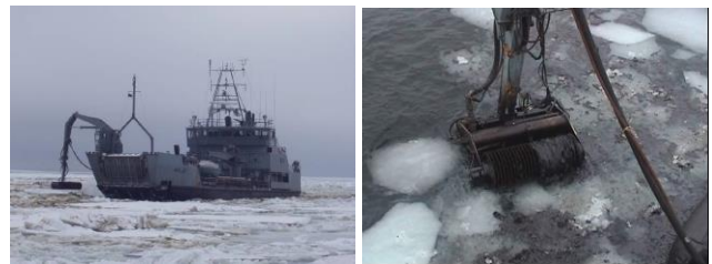
Fig.8 The spill response task by the vessel (left) and the oil recovery bucket in operation (right) in Finland.
